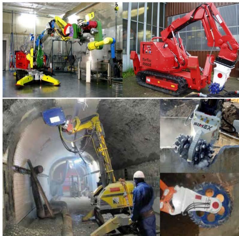
Figure 17: Optional equipment: dismantling device (top row: carrier with manipulator and tools, bottom row: with special tools for contouring, cutting etc.)
