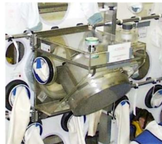
Fig: close up view of portholes equipped with gloves and with a lock-out system for 200L drums
