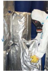
Manual preparation of new drums with outer liners to prevent contamination during filing
