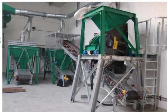
Example: Unit for safe collection of solid waste (soil, powders) from damaged packages
