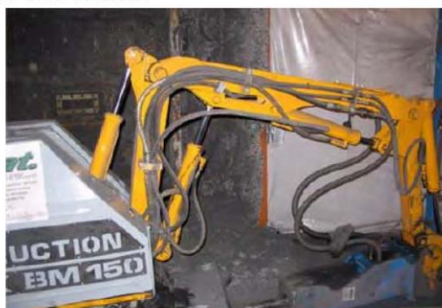
Example of electric excavator that can be used for recovering packages (Brokk 150)
