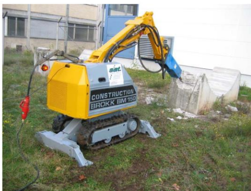
Example of sturdy electric-powered excavator for removal and handling of packages (here with pick)
