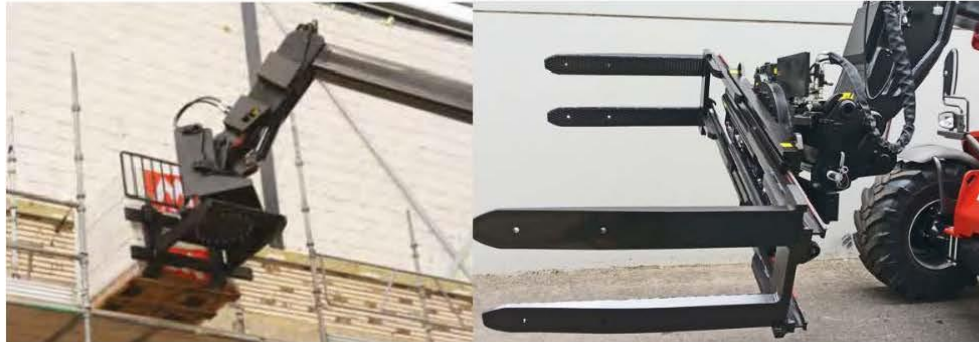
Figure 14: Useful accessories for telescopic handler: swing fork carriage (left) and rotator with grippers (right)
