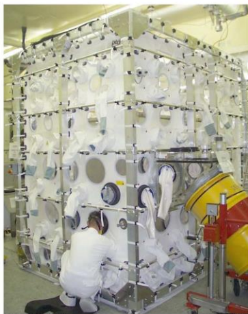
Fig: Example of tent for decontamination of highly contaminated objects in the nuclear industry
